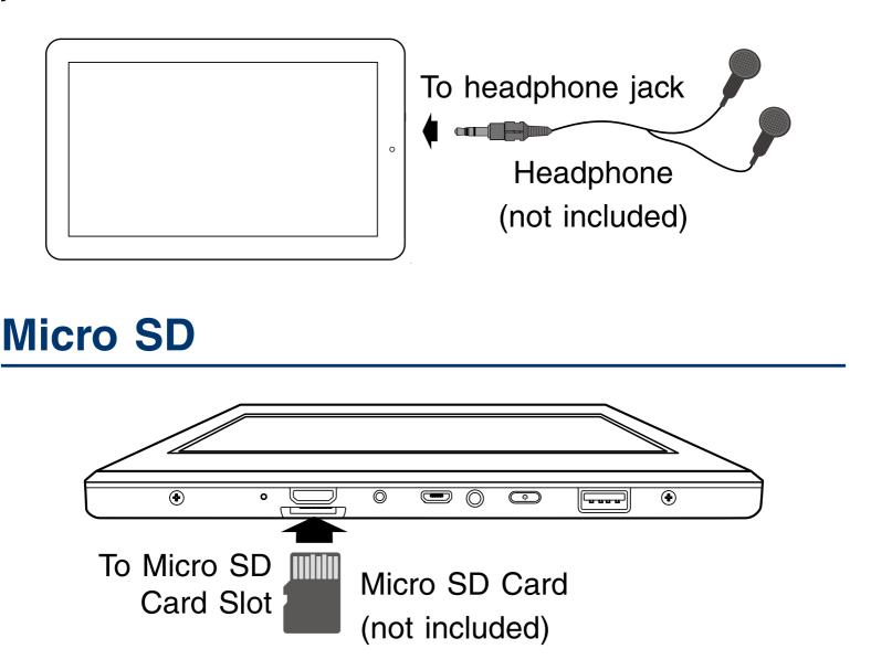
Insert the micro SD card into the tablet's Micro SD slot until it clicks.
